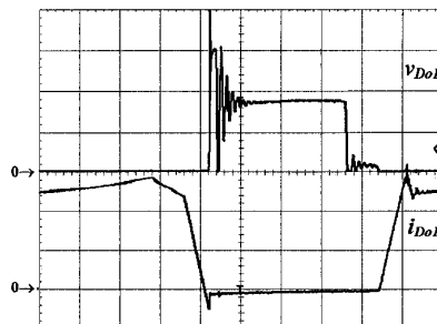
Fig. 10 – Experimental waveforms - diode D_{O1} . Upper trace: cathode-anode voltage v_{Do1} (100V/div. 2 \mu s/div.) Lower trace: anode current i_{Do1} (10A/div. 2 \mu s/div.)
