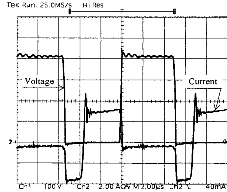
Fig. 11 – Current (2A/div) and voltage (100V/div) in one of the switches of the non-critical leg.
